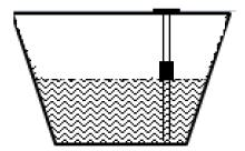
NOTE: Installation in cube or rectangle tanks can result in gauge readings that show ½ to ¼ less fuel than the actual fuel amount remaining (when the indicated level is showing less than half).
